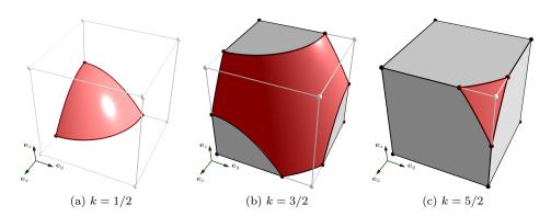
Fig. 5. Unit cube centred at  $\begin{bmatrix} 1/2 & 1/2 & 1/2 - k \end{bmatrix}^{\mathsf{T}}$  clipped by the elliptic paraboloid parametrically defined as  $z = -x^2 - y^2$ .
