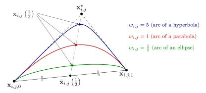
Fig. 4. Three rational Bézier arcs linking a start point  $\mathbf{x}_{i,j,0}$  to an end point  $\mathbf{x}_{i,j,1}$ . Also shown are the control point  $\mathbf{x}_{i,j}^{\star}$  and weight  $w_{i,j}$ , along with the points  $\bar{\mathbf{x}}_{i,j}\left(\frac{1}{2}\right)$  and  $\mathbf{x}_{i,j}\left(\frac{1}{2}\right)$  that can be used for determining  $w_{i,j}$ .
