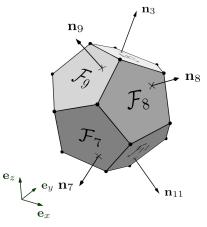
(b) The faces of  $\partial \mathcal{P} = \bigcup_i \mathcal{F}_i$  and their outwardpointing normal vectors,  $\mathbf{n}_i$ ,  $i \in \{1, \dots, n_{\mathcal{F}}\}$ .
