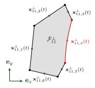
(c) Projected clipped face  $\hat{\mathcal{F}}_{11}^{\perp}$  and the splitting of its boundary into  $n_{\partial \hat{\mathcal{F}}_{11}} = 6$  parametrized arcs.
