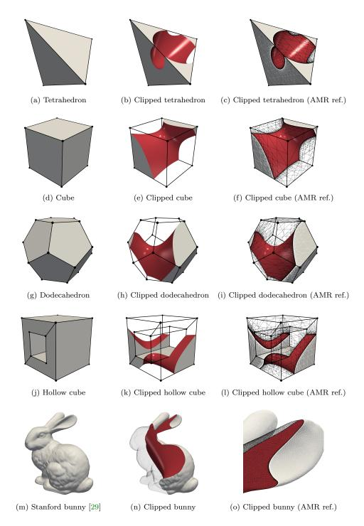
Fig. 7. Examples of random intersection cases between the five considered polyhedra and a paraboloid. The left column shows the full polyhedra; the central column shows the polyhedra clipped by a paraboloid; the right column shows the edges of the AMR of the polyhedra used for calculating the reference moments.
